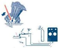
In this method the arc is established between a non-consumable tungsten electrode and the workpiece. The welder feeds a welding rod while operating the torch providing the protection gas with the other hand. This method produces superior quality seams and is particularly suited for root welding.
